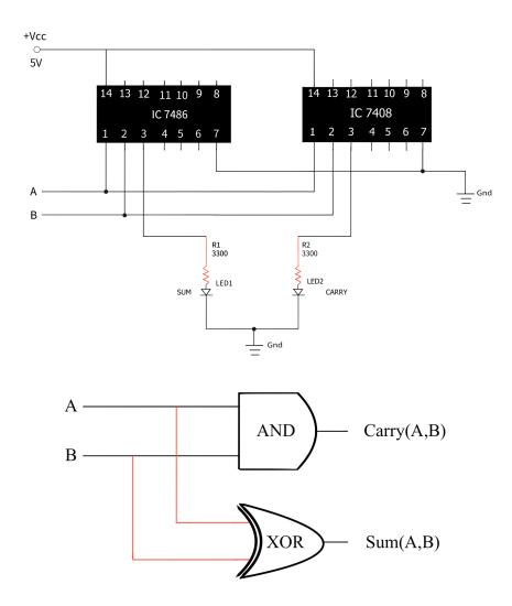
Figure 1: Below, the computational explanation (C) of a half-adder. On top is a possible implementation of it using integrated circuits (E); the outputs are delivered in terms of lights that can be on or off.
